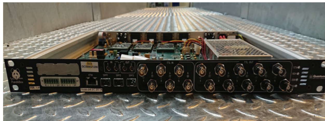
PandABox: Flexible triggering for continuous scanning.
