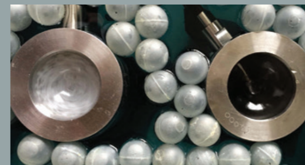
Figure 2: Two identical cooled, stirred wax solutions. The cell on the right is sonicated with specific low power ultrasound while the one on the left is not. The sample on the left crystallises as normal whereas nucleation is completely suppressed in the sonicated sample.
