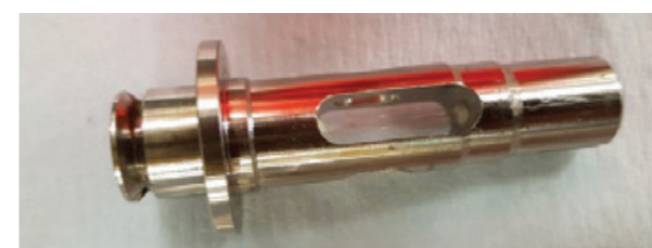
Figure 3: The capillary holder used on B21, with the atmospheric aerosol coating inside.
