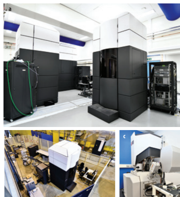
Figure 4: (a) eBIC Krios hall housing Titan Krios II, III and IV microscopes; (b) Titan Krios I located next to I20 in the experimental hall of Diamond; (c) the SCIOS cryo focused ion beam scanning electron microscope at eBIC.
